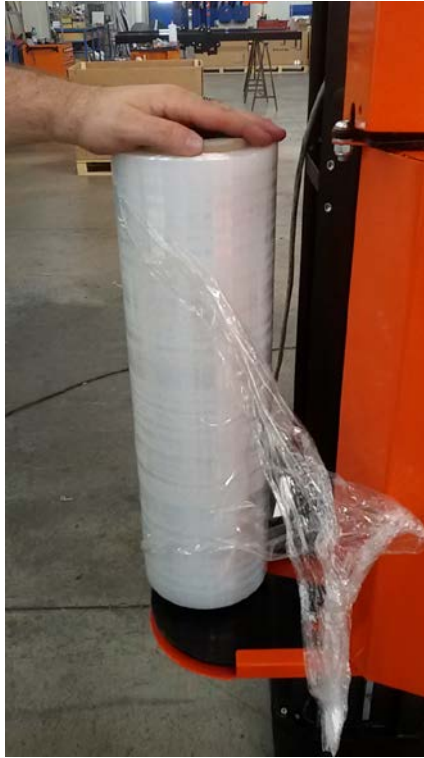
Phase 1: Insert the new film coil in the coil holder.
