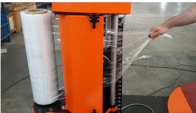
Phase 3 Pass the film end on the carriage rollers, as shown in the picture and close the door.
