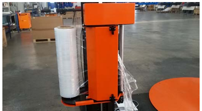
Phase 3 Pass the film end on the carriage rollers, as shown in the picture and close the door.
