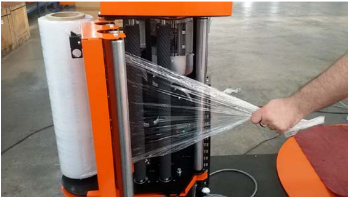
Phase 2: After opening the carriage door, pass the film end on the steel roller as shown in the picture. Pass the film end through the carriage rollers, as shown in the picture.
