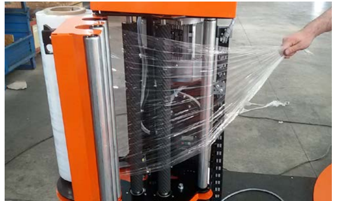
Phase 2: After opening the carriage door, pass the film end on the steel roller as shown in the picture. Pass the film end through the carriage rollers, as shown in the picture.
